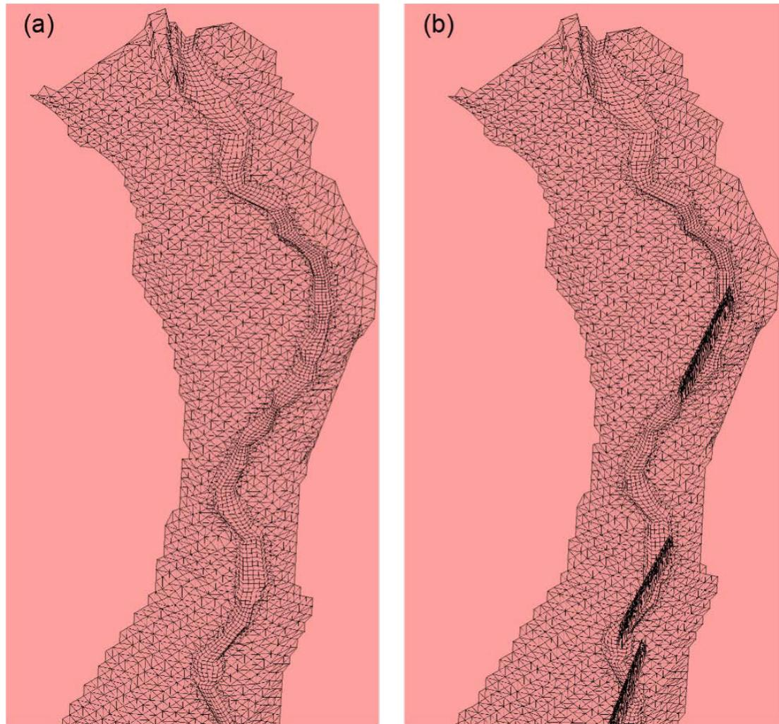
**Figure 3: (a) Calculation mesh of the hydrodynamic model used in simulation variants BV, V1 and V2 with the use of variable Strickler coefficients adjusted for the entire channel (V1) or adjusted at the positions of all LWD elements only (V2) and (b) mesh with discrete LWD elements used in variant V3. Example of the first 60 m of the study reach.**
