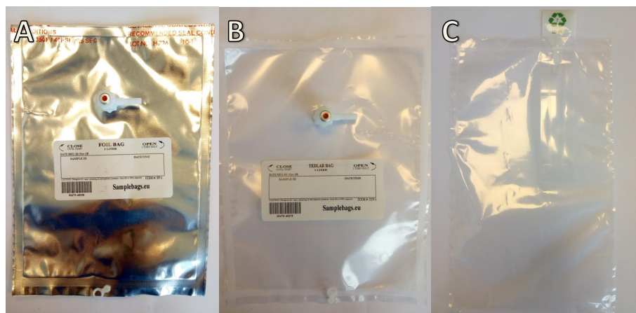
Figure A1. Sampling bags selected for the collection and storage of air. A is the methalized polyethylene (MPE) bag, B is the polyvinyl fluoride (PVF) bag and C is the low density polyethylene (LDPE) bag.
