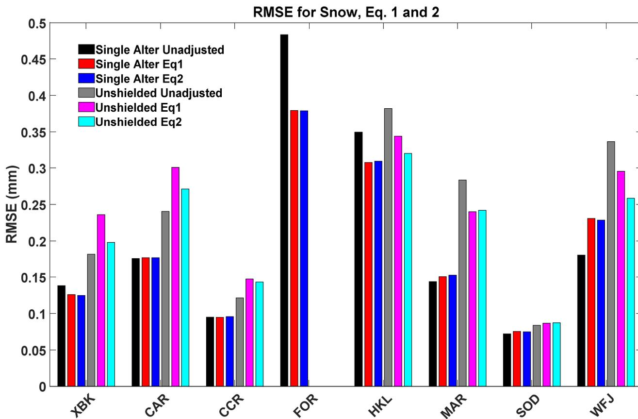
Figure 6: RMSE for snow for single-Alter and unshielded gauges for unadjusted measurements and for adjustments using Equations 1 and 2 at each of the eight SPICE sites, combining 2015/2016 and 2016/2017 winter seasons.
