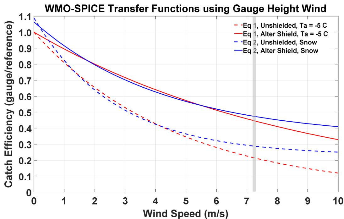
Figure 2. WMO-SPICE transfer functions from K2017b, Eq. 1 (red), Eq. 2 (blue) for unshielded (dashed), and single-Alter shielded (solid) gauges. Eq. 1 is plotted using an air temperature of  $-5^{\circ}\text{C}$  and Eq. 2 is plotted for snow. Both transfer functions are plotted for  $U_{gh}$  with the maximum wind speed threshold shown at  $7.2\text{ m s}^{-1}$ .
