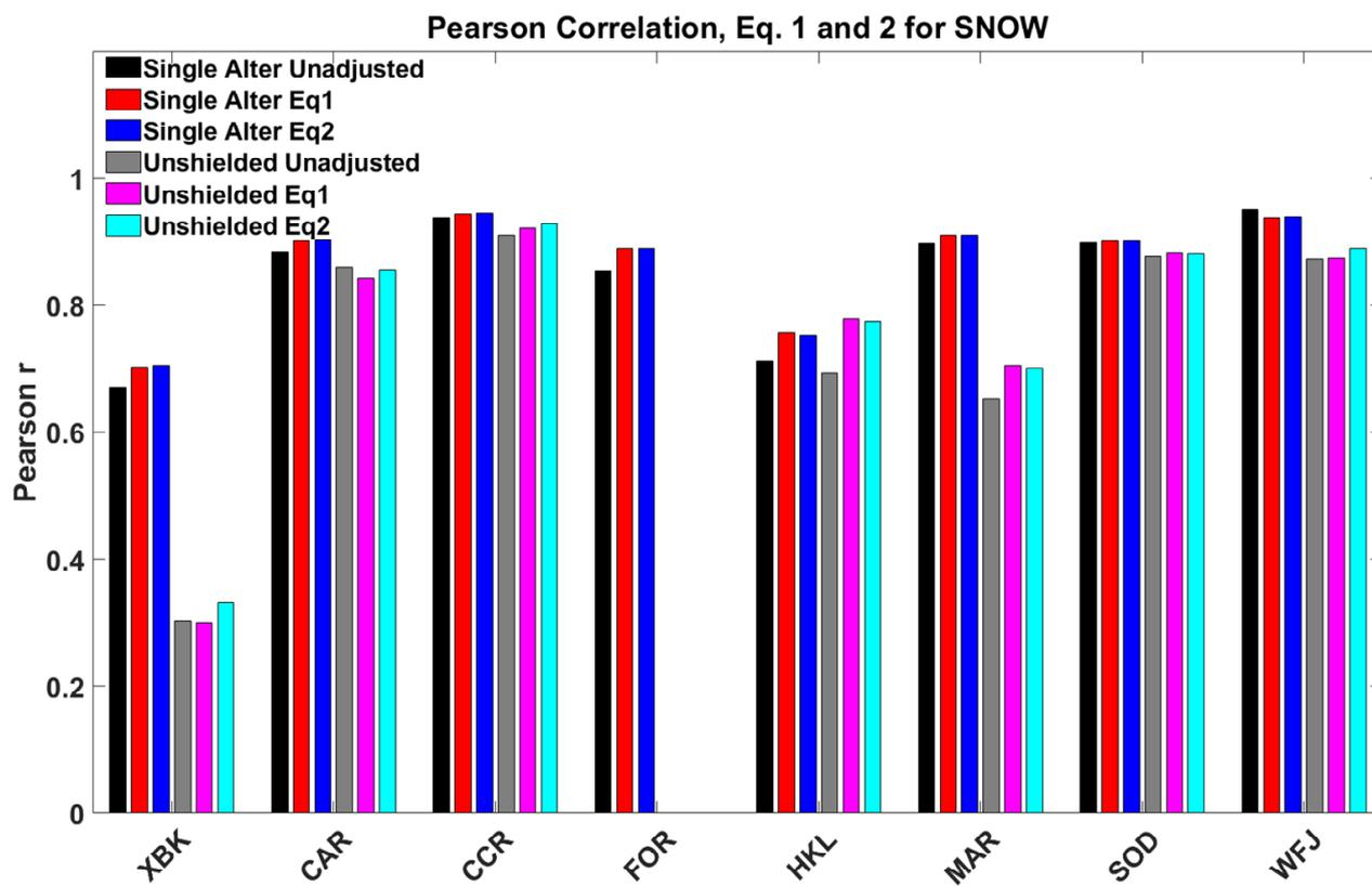
Figure 7: Pearson  $r$  for single single-Alter and unshielded gauges for unadjusted measurements and for adjustments using Equations 1 and 2 at each of the eight SPICE sites, combining 2015/2016 and 2016/2017 winter seasons.
