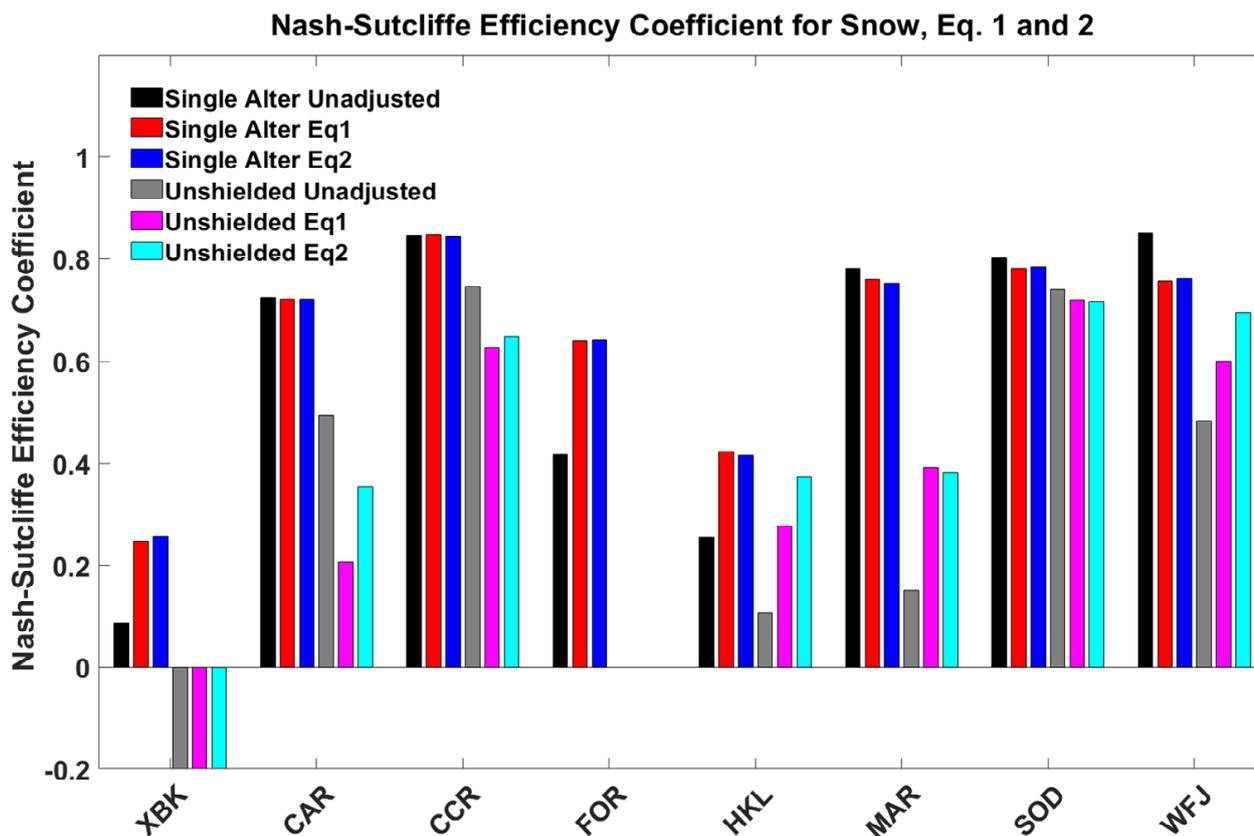
Figure 8: Nash-Sutcliffe Efficiency Coefficient for single single-Alter and unshielded gauges for unadjusted measurements and for adjustments using Equations 1 and 2 at each of the eight SPICE sites, combining 2015/2016 and 2016/2017 winter seasons.
