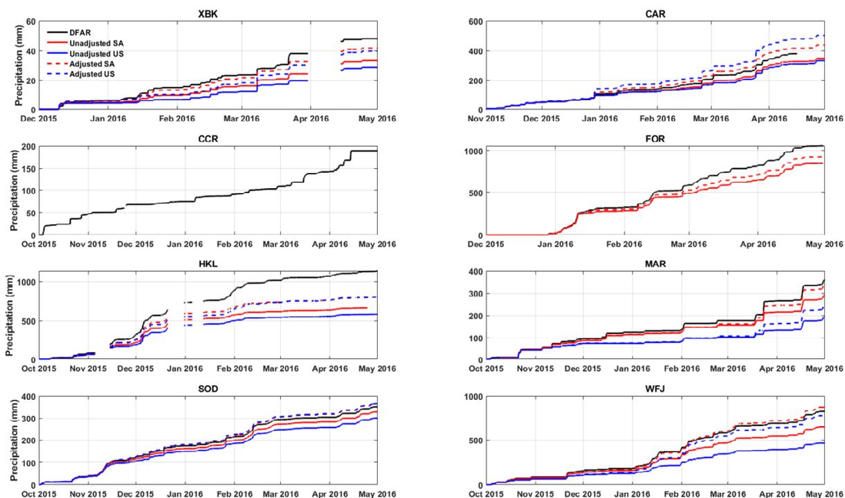
**Figure 3:** Time series of unadjusted (solid) and adjusted (dashed) precipitation time series for single-Altair shielded (red) and unshielded (blue) gauges as compared to the DFAR (black) during the 2015/2016 winter season at the eight SPICE sites.
