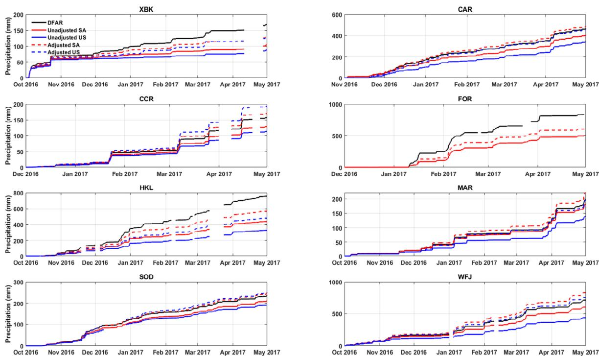
Figure 4: Time series of unadjusted (solid) and adjusted (dashed) precipitation time series for single- Alter shielded (red) and unshielded (blue) gauges as compared to the DFAR (black) during the 2016/2017 winter season at the eight SPICE sites.
