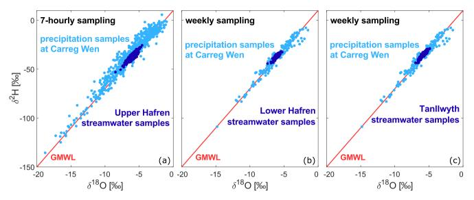
Figure 2: Dual-isotope plots for precipitation (light blue) and streamwater (dark blue) samples from 7-hourly (a) and weekly sampling (b-c). Both precipitation and streamwater samples generally fall close to the global meteoric water line (GMWL, red line), and thus show little evidence of evaporative fractionation.
