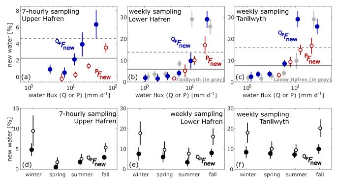
Figure 10: Event new water fractions  $\binom{Q_p}{F_{new}}$  and new water fractions of precipitation  $\binom{P}{F_{new}}$  for different discharge rates, precipitation rates, and seasons, calculated from time series of oxygen-18. Error bars indicate one standard error. In panels (a)-(c), solid circles indicate event new water fractions, plotted as functions of discharge rates, and open circles indicate new water fractions
