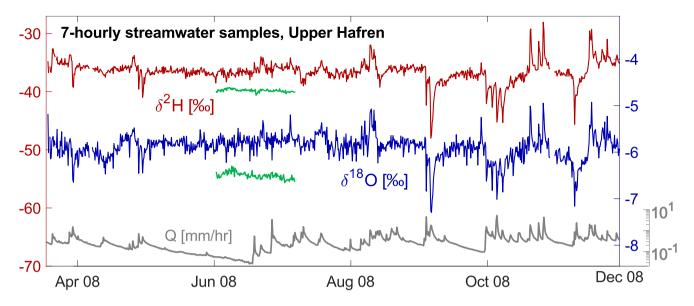
Figure 6: A close-up of the 8 months of nearly complete streamwater samples from 7-hourly sampling. Deuterium (left axis) is shown in red, oxygen-18 (right axis) in blue, and discharge is shown in gray. The fluctuations of the replicate QC standards from the reproducibility test (green) illustrate the magnitude of the variability between samples due to analytical noise.
