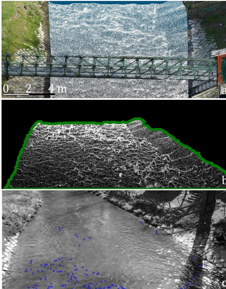
Figure 3: Defining the search area to extract particles to track. a) 3D point cloud of the investigated river reach at the Wesenitz. Coloured points (colorized with RGB information according to their real world object colour) are 3D points above the water surface reconstructed with SfM photogrammetry. White points are 3D points below the water surface reconstructed with SfM and corrected for refraction effects. b) 3D point cloud below the water level projected into image space. Green line depicts contour line, which is used as search mask for feature detection. c) Detected and filtered features considered for tracking (blue circles). 585
