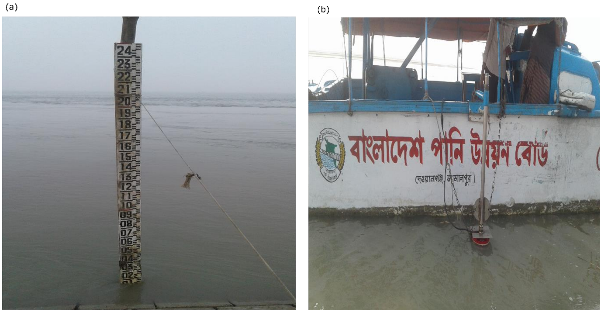
Figure S1: (a) Water level staff gauge at Bahadurabad gauging station; (b) Discharge measurement using the ADCP Bahadurabad gauging station, Brahmaputra river in Bangladesh (Photo credit: Hydrology division, BWDB)
