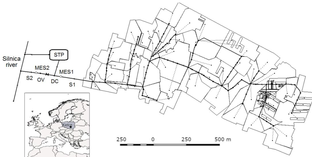
Figure 1: Diagram of the analysed urban catchment.
