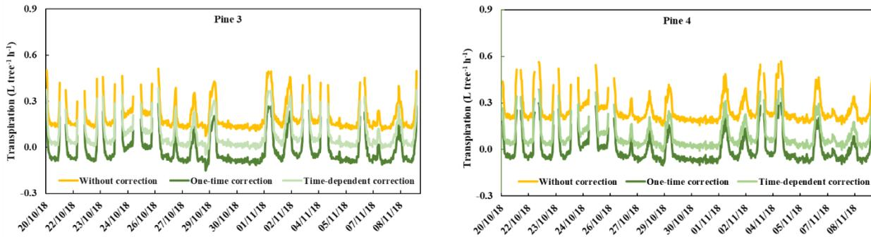
Figure 7. Three weeks of transpiration rates ( $L \text{ tree}^{-1} \text{ h}^{-1}$ ). ‘Without correction’ represents rates without misalignment-corrections, ‘One-time correction’ represents rates corrected for once in the beginning of the measurement period, and ‘Time-dependent correction’ represents rates being corrected for at varies days throughout the measurement period.
