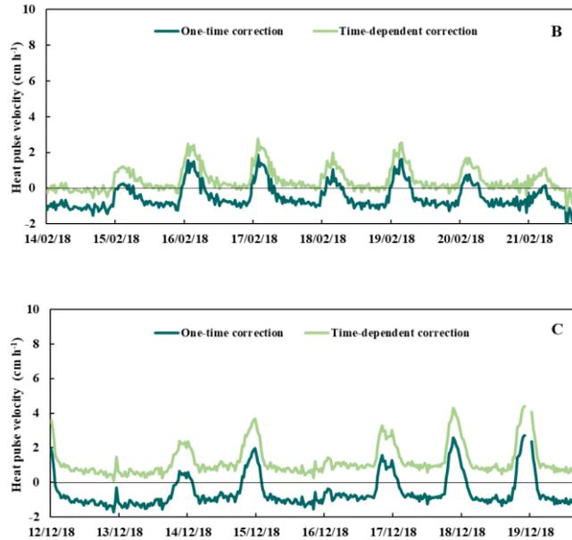
290 Figure 5. Heat pulse velocities during one week of measurements in the beginning (A), halfway (B) and at the end (C) of the measurement period. Dark green lines represent velocities with probe misalignment corrected for once at the beginning of the experiment. Light green lines represent velocities with the time-dependent probe misalignment corrections.
