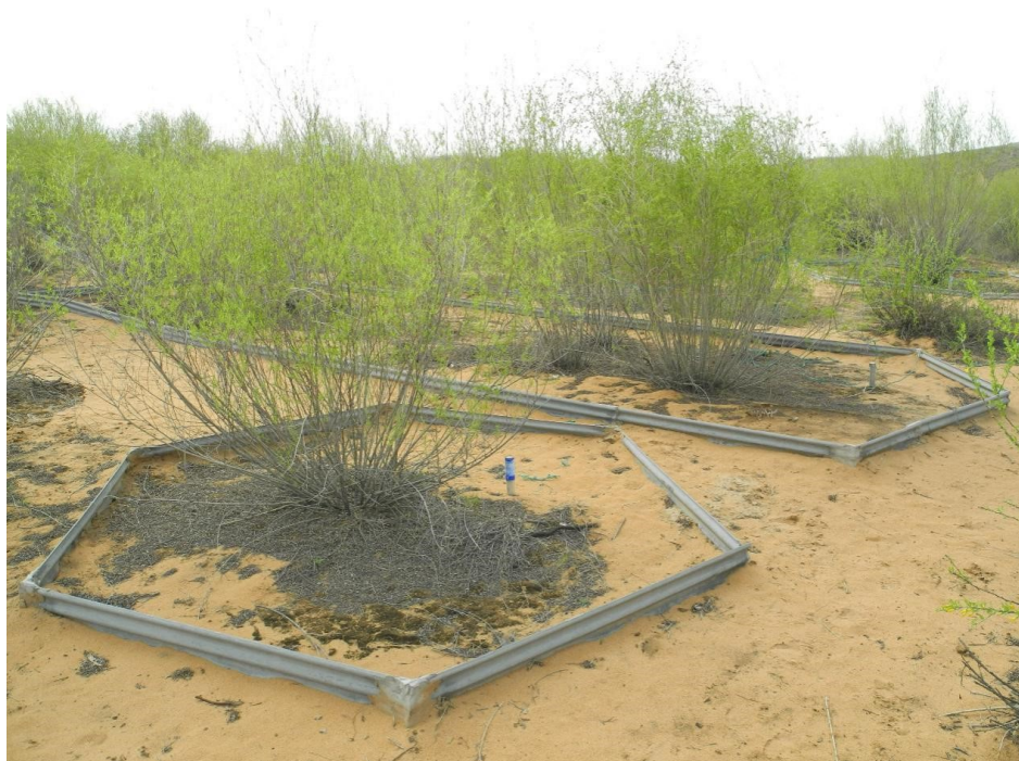
Fig. 1. Fig. R2-1. The established runoff and sediment plots at the S. psammophila plot.
