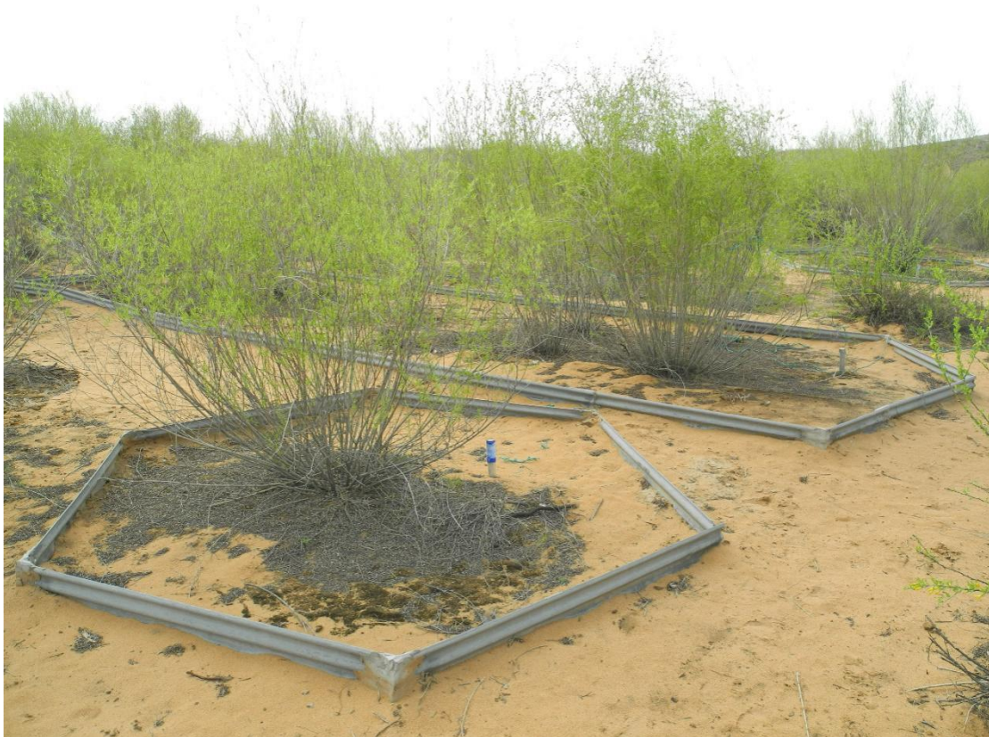
Fig. R2-1. The established runoff and sediment plots at the S. psammophila plot. (4) Stemflow intensity had been re-calculated on the basis of branch basal area. Please see the detailed description at Point (1) of Reply to R2C2 .
