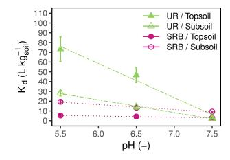
**Figure 3.**  $K_d$ -values as function of pH for UR (triangles, dash-dotted lines) and SRB (circles, dotted lines) in topsoil (filled symbols) and subsoil (open symbols). Each  $K_d$ -value was derived as the slope from linear regression of the sorption isotherms (six concentrations times three replications). The error bars represent the standard errors of  $K_d$ -values from linear regression.
