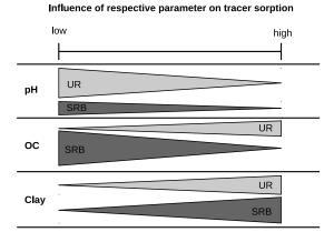
Figure 7. Schematic figure of the influence of the parameters OC, Clay and pH on the adsorption of the fluorescent tracers UR and SRB.
