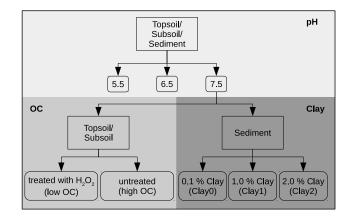
Figure 1. Experimental design for the different treatments of the batch experiments.
