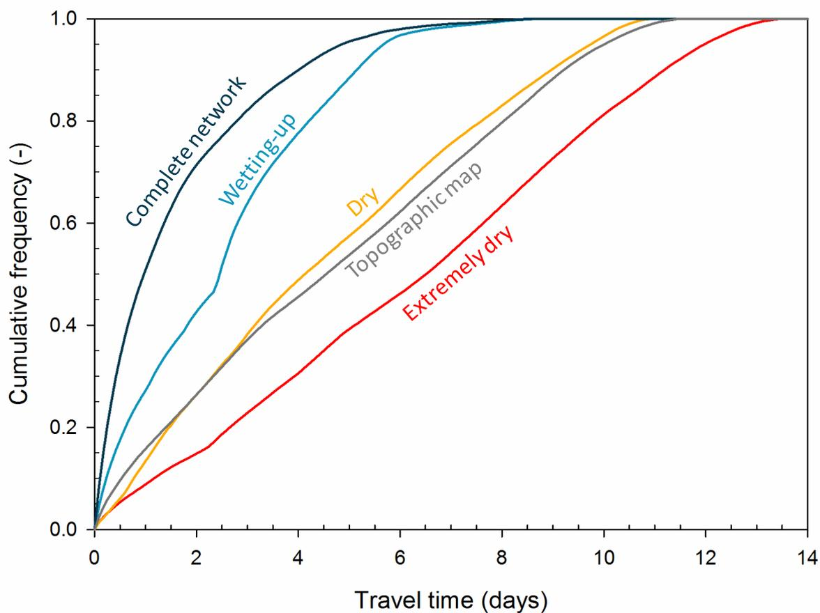
Figure 5. Cumulative frequency distributions of the travel time ( $t_i$ ) to the catchment outlet for the five flowing stream networks shown in Figures 2 and 4. See Table 2 for the main descriptive statistics of the travel time distributions.
