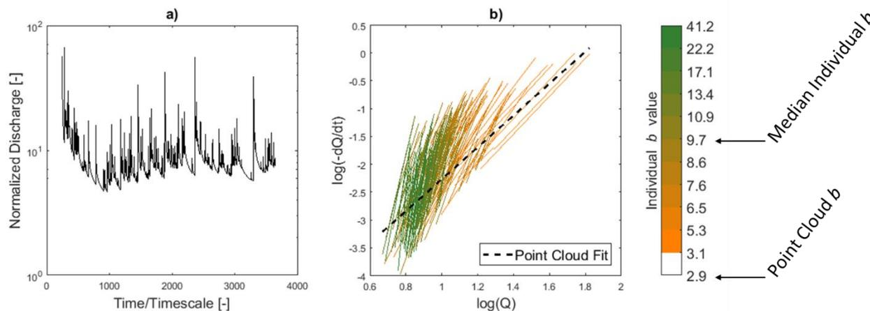
**Figure 6.** a) Hydrograph with lognormal distribution in recharge event inter-arrival times and magnitudes, and b) recession analysis plot showing a large range of  $b$  values (with the median of  $b = 9.7$ ), compared to the point cloud fit (black dotted line-BA  $b = 2.9$ ). The color bar is divided into deciles in the distribution of  $b$  values compared to the point cloud range.
