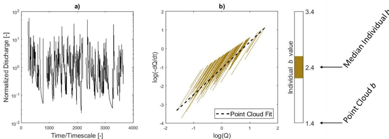
**Figure 4.** a) Hydrograph with log-normally distributed event inter-arrival times and peak magnitudes with each event maintaining a constant falling limb decay constant, and b) recession analysis with resulting parallel individual recessions having a constant  $b$  value (MI  $b = 2.4$ ) compared to the point cloud fit (black dotted line) which results in  $b = 1.4$ ). The individual recessions are offset which when viewed collectively, results in the point cloud.
