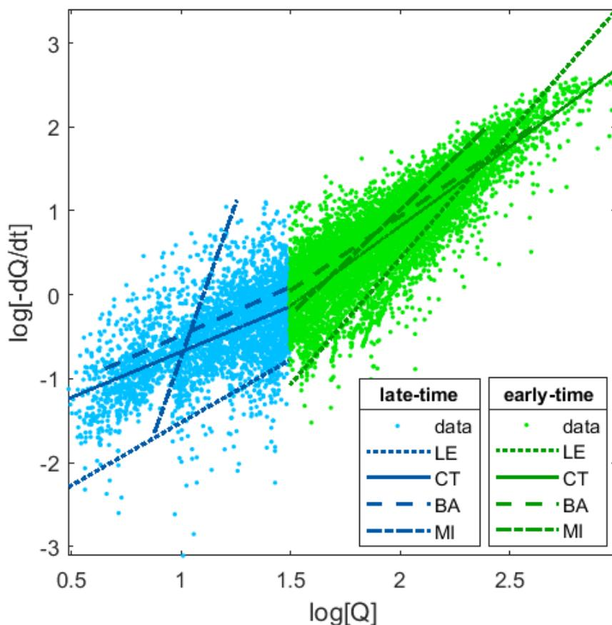
**Figure 3.** Recession analysis for Lookout Creek to aid in the comparison of four different fitting methods and the dependency on parameter estimation shown visually (lower envelope (LE), central tendency (CT), binning average (BA)) and individual recessions parameters (median individual recession (MI)). Depending on the fitting method, the parameter estimation for  $a$  and  $b$  will be different.
