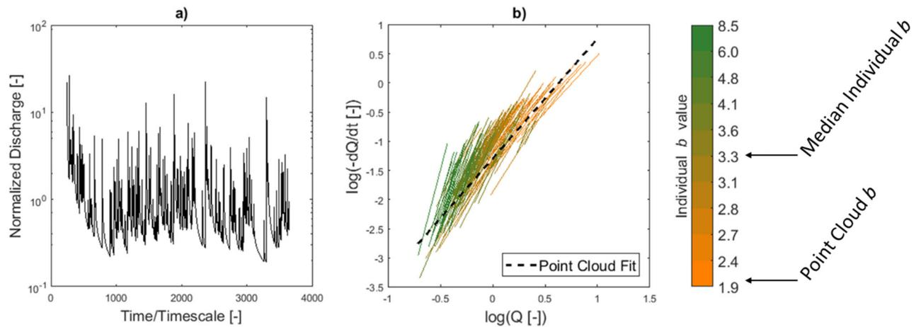
**Figure 6.** a) Hydrograph with lognormal distribution in recharge event inter-arrival times and magnitudes, and b) recession analysis plot showing a large range of  $b$  values (with the median of  $b = 3.3$ ), compared to the point cloud fit (black dotted line- BA  $b = 2.0$ ). The color bar is divided into deciles in the distribution of  $b$  values compared to the point cloud range.
