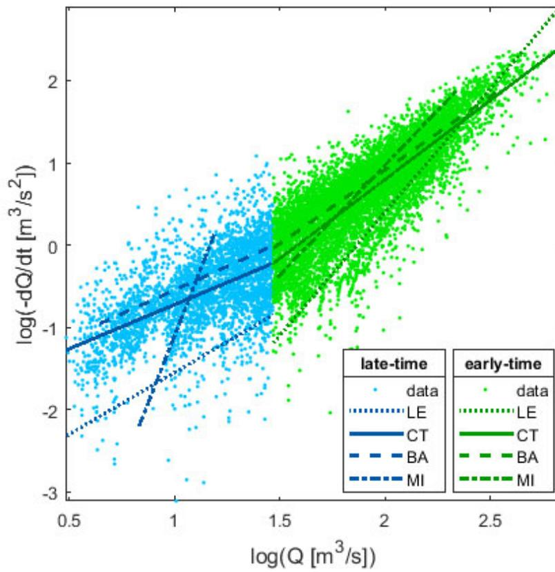
**Figure 3.** Recession analysis for Lookout Creek to aid in the comparison of four different fitting methods and the dependency on parameter estimation shown visually (lower envelope (LE), central tendency (CT), binning average (BA)) and individual recessions parameters (median individual recession (MI)). Depending on the fitting method, the parameter estimation for  $a$  and  $b$  will be different.
