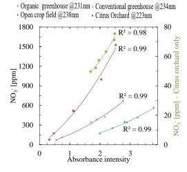
Figure 8: Calibration equations for the four study sites. As can be seen on the chart legend, each of the sites has its own unique optimal wavelength for estimating nitrate concentration. Note that the right ordinate shows a lower concentration range than the left ordinate and is associated only with the citrus orchard.
