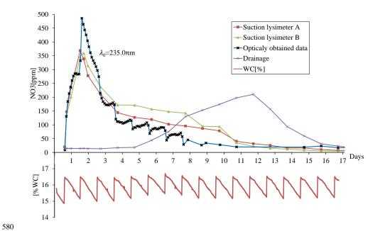
Figure 10: Breakthrough curves plotted for physically sampled solution and calculated nitrate concentration, as obtained automatically by the optical setup. The bottom curve shows the soil water content as obtained by the water-content sensor (TDT).
