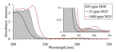
Figure 1: Absorption spectra of nitrate at concentrations of 25 ppm, 1000 ppm, and 5 ppm dissolved organic carbon (DOC).
