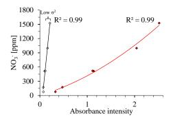
Figure 7: Calibration curves created using absorbance data at 238 nm and 300 nm.
