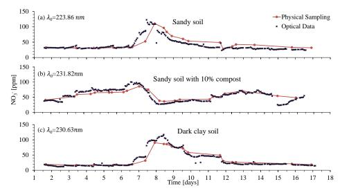
Figure 11: Nitrate breakthrough curves for (a) sandy soil, (b) sandy soil with 10% compost and (c) dark clay soil.
