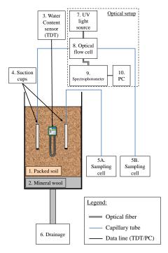
555 Figure 2: Soil-packed column and optical setup for nitrate breakthrough curve experiment.
