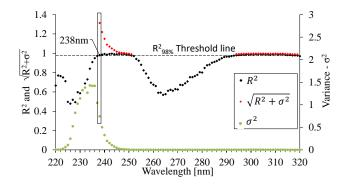
Figure 6: Relationship between coefficient of determination ( $R^2$ ), variance ( $\sigma^2$ ) and the UV spectrum for the open crop field.  $\sqrt{(R^2+\sigma^2)}$  was calculated only for values where  $R^2$  exceeded the set threshold at  $R^2$ <sub>98%</sub>. The maximum calculated value was determined as the optimal wavelength and was set to 238 nm.
