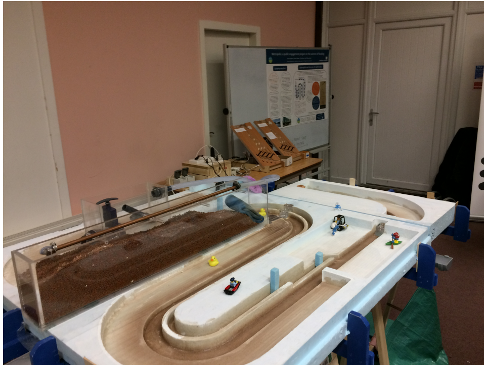
Figure 8. Photograph of the entire set-up at the Churchtown Flood Action Group workshop on 28-01-2017, with the winding river channel in the foreground, the city plain with a few smurfs, the groundwater moor, the reservoir on the left behind the moor, and in the background on the right, the control table with the Arduino units and the two Galton boards as well as an informative poster on Wetropolis.
