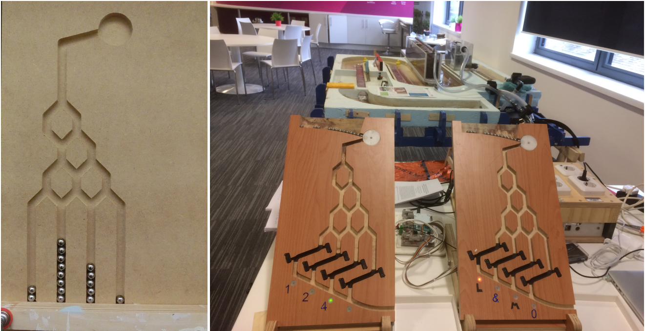
Figure 1. Photographs of asymmetric Galton boards. Test board on the left and a final set-up on the right. At every split the chance of a steel ball falling to the left or right is 50% for a well-balanced Galton board. When a sufficiently large number of steel balls falls through this Galton board, the discrete distribution becomes (3, 7, 5, 1)/16 . The 4 \times 4 possible outcomes in two of such boards, registered in each by four electronic eyes (located in the black-painted areas along 2 \times 4 = 8 channels marked here by “1, 2, 4, ...” and “L, &, M, 0”), determine both the rainfall amount and its location(s) in Wetropolis. The outcome of the random draw, shown by the lit-up lights, will in this instance lead to 4s of rain in the lake/reservoir. Photos: OB & WZ.
