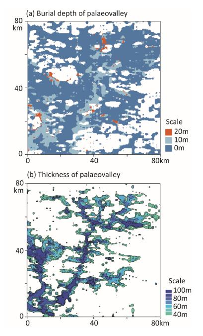
400 Figure 11: (a) Burial depth and thickness (>40 m) of the alluvium sediments in palaeovalleys inferred from the 3D binary valley image of Fig. 9c with a 10-m vertical resolution. The hollow zone in (a) represents no identified palaeovalleys within the depth of 100 m in the study area.
