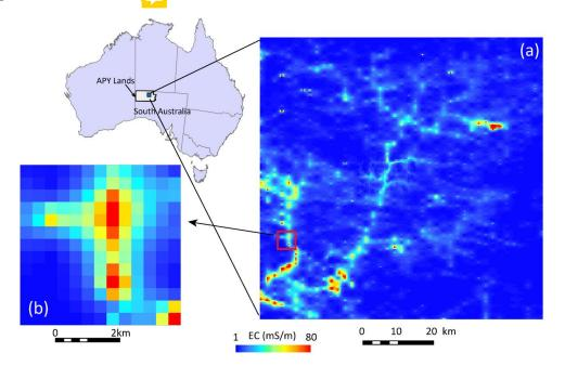
Figure 1: (a) Electrical conductivity at 100 m depth ranging from 1 to 80 mS/m (1 mS/m=0.01 dS/m) as interpreted from airborne electromagnetic surveys in the Anangu Pitjantjatjara Yankunytjatjara (APY) Lands, Australia; (b) inset shows detail of EC map at a spatial resolution of 400 × 400 m (Soerensen et al., 2016).
