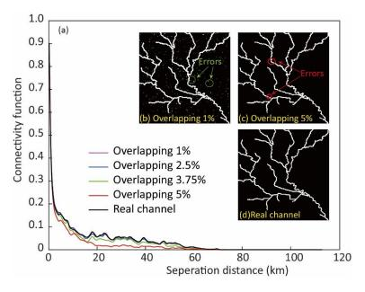
Figure A3: (a) Connectivity function in the northwest to southeast direction when applying the trained SRCNN to generate synthetic palaeovalleys. Resultant palaeovalley patterns using trained SRCNN with various degrees of overlap (1% (b) and 5% (c)) in comparison with real palaeovalley (d).
