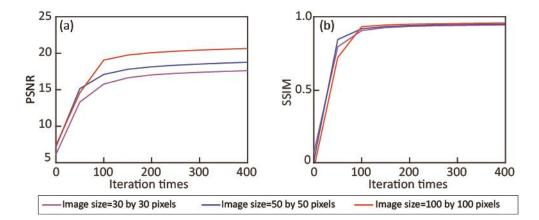
Figure A4: Performance criteria PSNR (a) and SSIM (b) calculated by the SRCNN for the testing dataset under varying input
