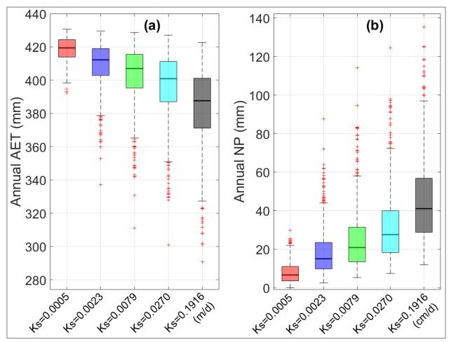
Figure 14: Box plots showing the distribution in variability in the simulated water balance components of (a) AET and (b) NP with variation in the soil hydraulic parameters, for instance, Ks of the LOS overburden. Variability of each water balance component is represented for the five illustrative covers. Description of the box plots is the same as for Fig. 11.
