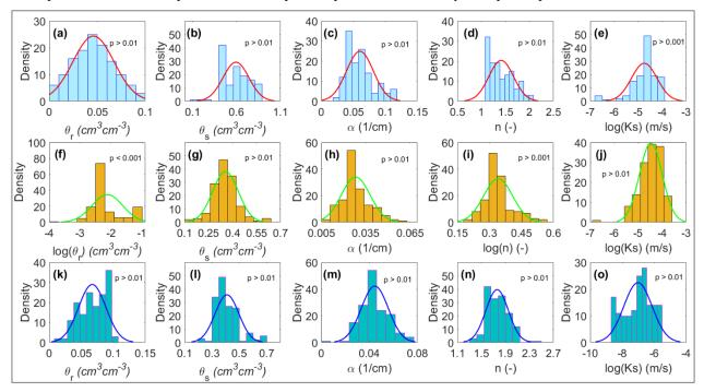
Figure 3: Probability density functions (PDFs) fitted to the four VG parameters and Ks obtained from the IM for the three soil types: peat (a-e), subsoil (f-j), and LOS (k-o). The mean and SD of the fitted distributions are shown in Table 2.
