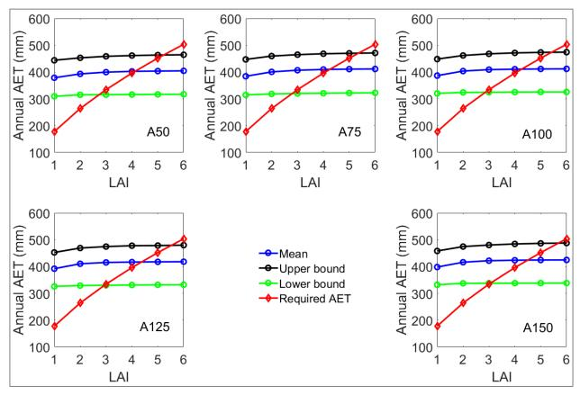
Figure 10: Lower (10%), mean, and upper (90%) limits of LAI\_max values for the five illustrative covers showing variability in the LAI values based on the simulated annual AET with the 700 parameter sets over a 60-year climate cycle.
