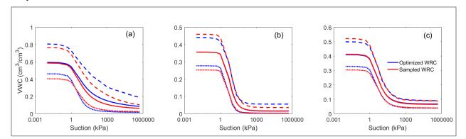
Figure 6: Estimated mean (solid lines) with 10<sup>th</sup> (dotted lines) and 90<sup>th</sup> (dashed lines) percentiles of the soil water retention curves (WRCs) for (a) peat, (b) subsoil, and (c) LOS obtained from the 155 optimized and 700 randomly sampled parameter values, where VWC denotes volumetric water content.
