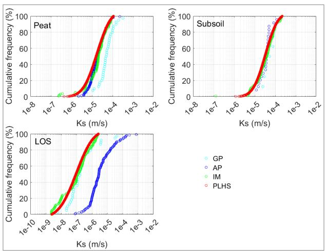
Figure 7: Comparison of the cumulative frequency distributions of the field-measured Ks using GP and AP methods, and optimized (IM) Ks values with the randomly sampled (PLHS) 700 Ks values. The results shown are for peat, subsoil, and LOS soil types.
