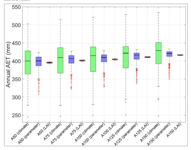
Figure 12: Box plots showing the distributions of annual AET obtained from the simulated water balances for the five illustrative covers with 700 parameter sets (blue boxes show parameter variability) over a 60-year climate cycle (green boxes
