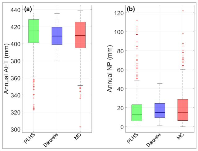
Figure 15: Box plots showing the distributions of (a) annual AET and (b) annual NP obtained from the simulated water balances for A100 illustrative cover with 700 parameter sets for PLHS (green boxes), 135 parameter sets for discrete sampling (blue boxes), and 1000 parameter sets for MC (red boxes) over a 60-year climate cycle. Description of the box plots is the same as for Fig. 11.
