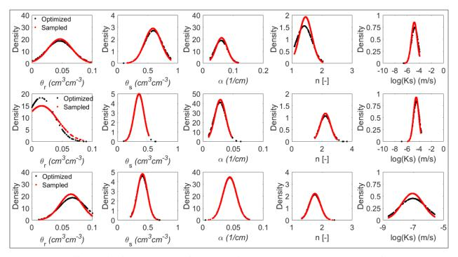
Figure 5: Probability density functions (PDFs) for the optimized and sampled 700 parameter sets for the peat coversoil (top row), subsoil (middle row), and LOS (bottom row).
