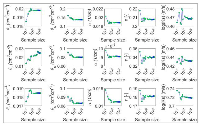
Figure 8: (a) Mean and (b) SD of the sampled parameter values corresponding to each sample size. Results are shown for peat (top row), subsoil (middle row), and LOS (bottom row) in both (a) and (b).
