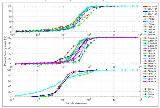
Figure 2: Particle size distribution for peat (peat/LFH/GBLFH), subsoil (subsoil/CBM/TBOB/GBBM), and LOS (CS) materials (OKC, 2009)
