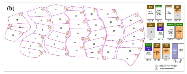
Figure 1: (a) Location map of Aurora North Mine of Syncrude Canada Ltd. and (b) soil cover design treatments (TRT) at ASCS (adapted from OKC, 2017). LOS overburden (OB) underlies all treatments, even though treatments with less than 150 cm total soil cap thickness only show OB
