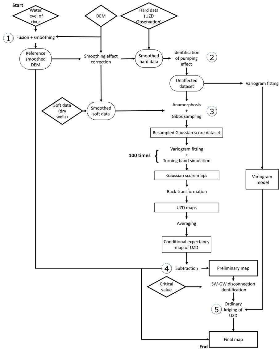
**Figure 1.** Flow chart for the mapping of water table. Steps 1 to 4 for first guess map. Step 5 for the final map. UZD: unsaturated zone depth. Diamonds display raw data, ellipses display input data after pre-processing and squares display intermediary products.
