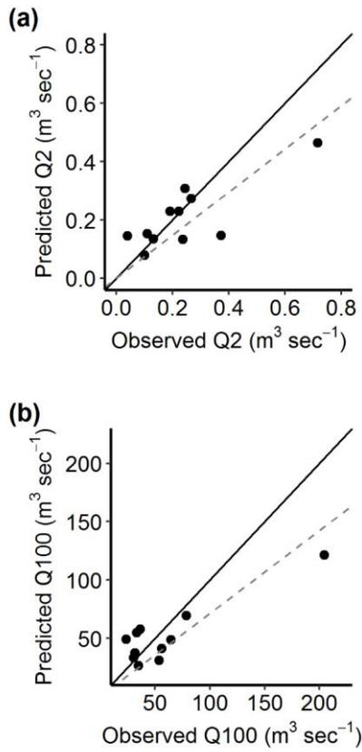
1294 **Figure 2** – Observed versus predicted estimates for (a) Q2, and (b) Q100. The dashed grey line
