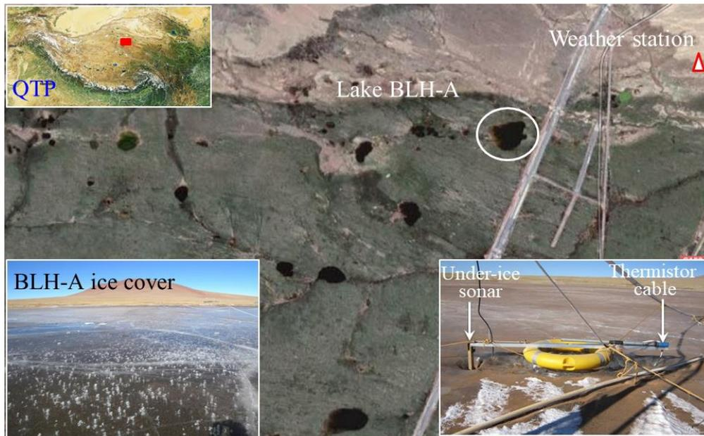
**Figure 1.** Location of Lake BLH-A. The lower left insert photo shows the lake ice cover including numerous large bubbles, while the lower right insert shows field instrumentation for temperature and ice thickness measurements. Thin deposited fine sand film (dark yellow) is also seen in both inserts.
