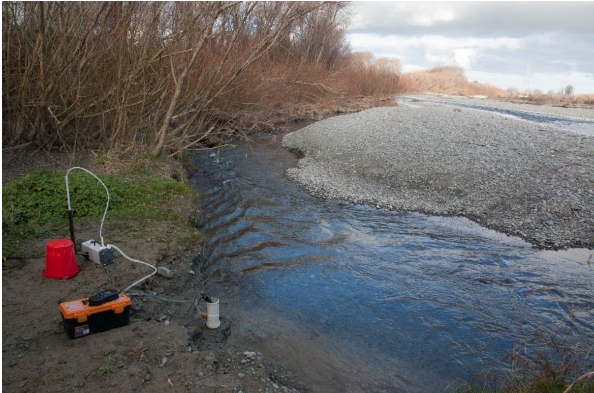
479 Figure 5. Mini-piezometer installed on the bank of a braided river (Coluccio, 2018).
