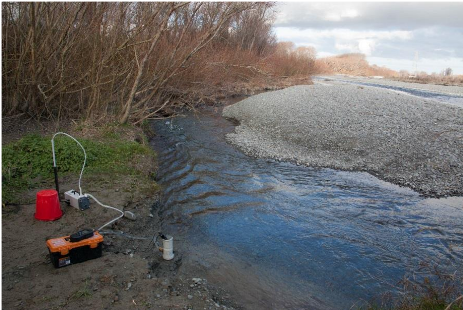
489 Figure 5. Mini-piezometer installed on the bank of a braided river (Coluccio, 2018).
