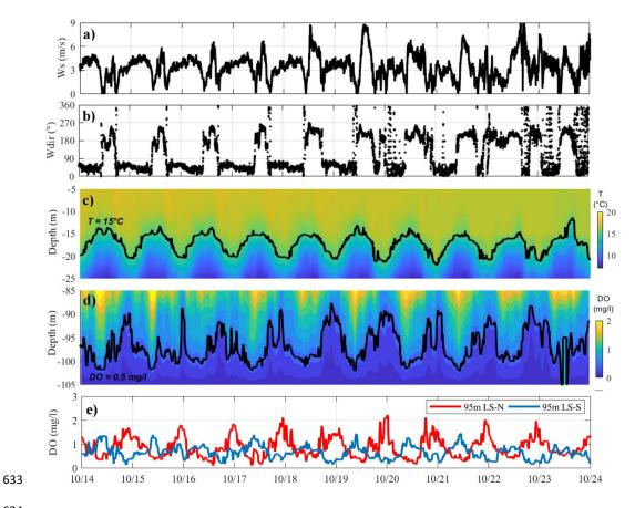
**Figure 4.** Time series measured from 14 to 24 October 2017 of (a) wind speed and (b) direction at LS-N, followed by the spatial and temporal variation of (c) temperature between 5 and 25 m at LS-N and of (d) dissolved oxygen between 80 and 105 m at LS-S. Panel (e) compares the time series of DO measurements at LS-N and LS-S stations. In correspondence of each tick of the horizontal axis it is 00:00 o'clock.
