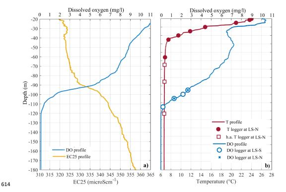
**Figure 2.** (a) Vertical profile of normalized conductivity (EC25) and dissolved oxygen (DO) measured on 10/04/2018 at the LS-N. (b) Vertical profile of temperature (T) and dissolved oxygen (DO) measured on 22/07/2017 at the LS-N. The circles and the crosses show the location of the dissolved oxygen sensors at LS-S and LS-N, respectively. The dots and the squares show the location of the temperature sensors at LS-N, with the squares indicating the high accuracy sensors.
