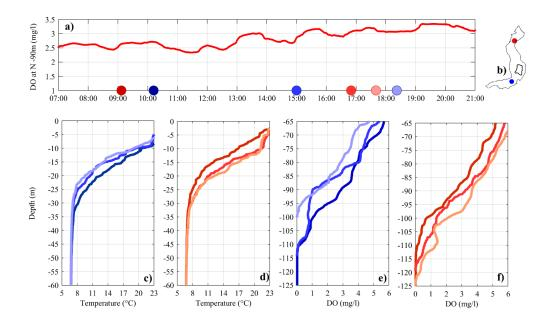
**Figure 7.** (a) Dissolved oxygen (DO) concentration at 90 m depth recorded at station LS-N on 21 July 2017. Coloured dots on the x-axis indicate the sampling time of the vertical profiles shown in the panels (c-f). Panels (c) and (d) compare the profiles of temperature between 0 and 60 m, while panels (e) and (f) compare the profiles of DO between 65 and 125 m. Red and blue colours refer to the northern and southern sampling location (see panel b), respectively.
