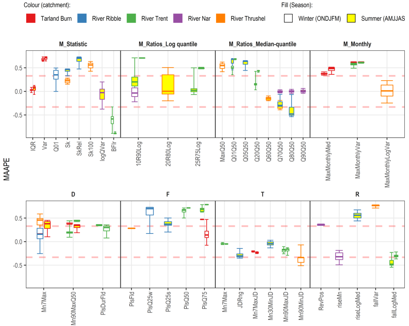
Figure 4. Mean arctangent absolute percentage error (MAAPE) values for each ER HI. As per HAF, the acceptable range is defined as \pm 0.33 (red dashed line). The 4- and 5-parameter results are adjacent, left and right respectively, for the Tarland Burn and River Trent.
