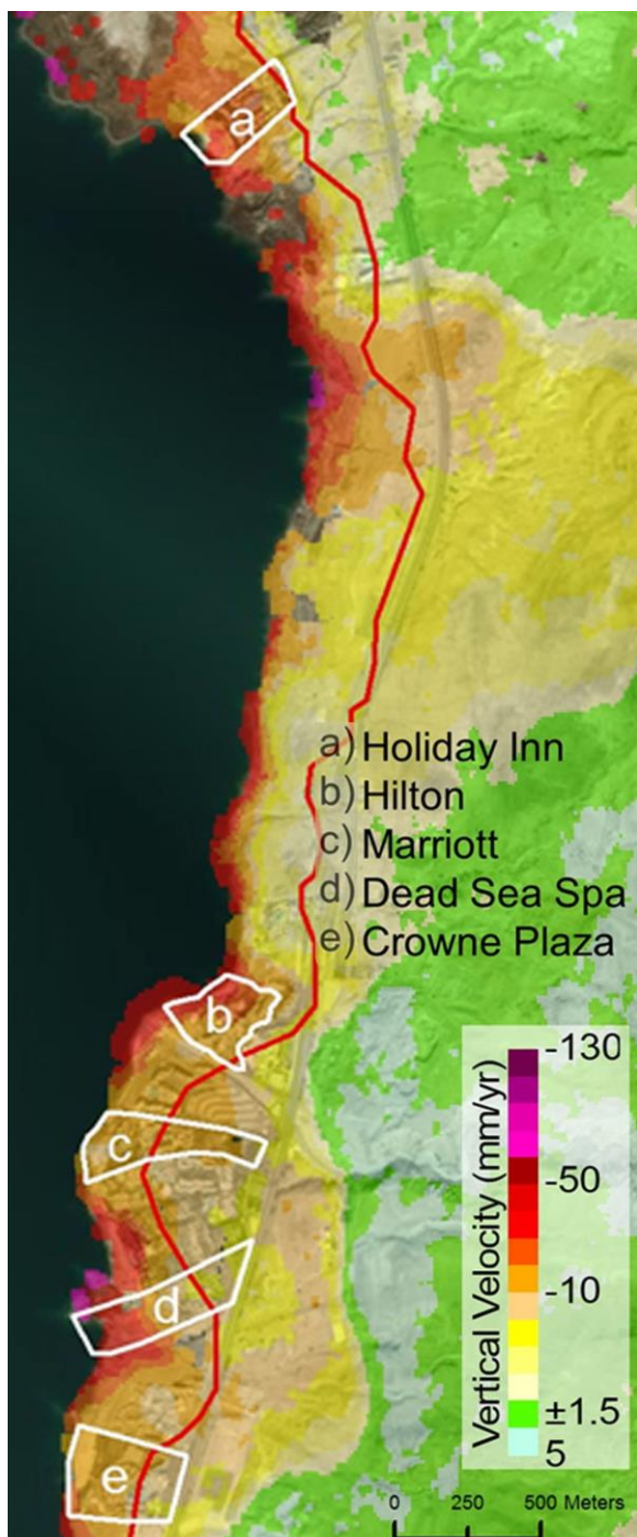
Figure 4: vertical velocity map of the study area obtained from the SBAS processing of Sentinel-1A/B images. The red line indicates the shoreline in 1959.
