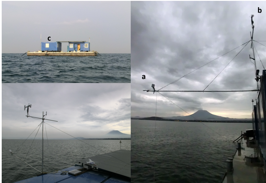
Figure 2. Automatic weather station on Lake Kivu after its installation, 8 October 2012 (©Wim Thiery). a indicates the location of the temperature, relative humidity and radiation sensors at 4.40m above the lake surface. b shows the location of the wind vane at 7.20 m above the lake surface. c indicates the container on which the station was mounted.
