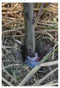
**Changes in the manuscript**: Added a sentence in line 126 'To sample porewater from the clay, we used the open auger boring method (De Goffau et al., 2012). We drilled a hole with a hand auger, without any drilling fluid. Then we waited for the hole to fill with water, which we sampled by inserting a sample bottle into the hole with a
