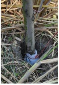
Changes in the manuscript: Added a sentence in line 126 'To sample porewater from the clay, we used the open auger boring method (De Goffau et al., 2012). We drilled a hole with a hand auger, without any drilling fluid. Then we waited for the hole to fill with water, which we sampled by inserting a sample bottle into the hole with a stick, which we pulled back out using a rope that was attached to the bottle.' Changed the name of these samples from 'hand-auger borings' to 'open auger borings'
