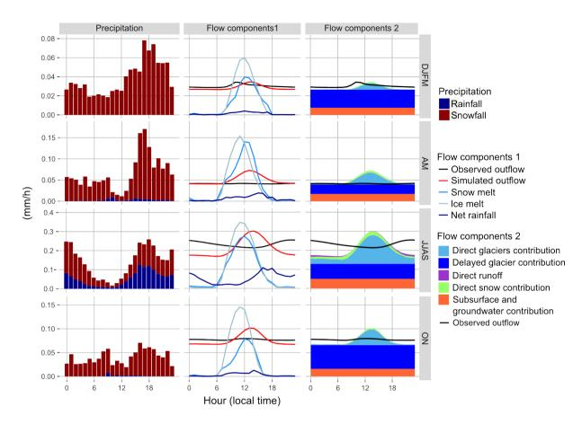
**Figure 15.** Mean hourly precipitation, discharge and flow components simulated with configuration v3 and averaged for the winter (DJFM), pre-monsoon (AM), monsoon (JJAS), and post-monsoon (ON) seasons. Note different y-axis scales for each season
