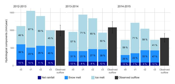
Figure 7. Simulated annual hydrological contributions (Definition 1) to Pheriche outflow for 3 glaciological years from 12/2013 to 11/2015
