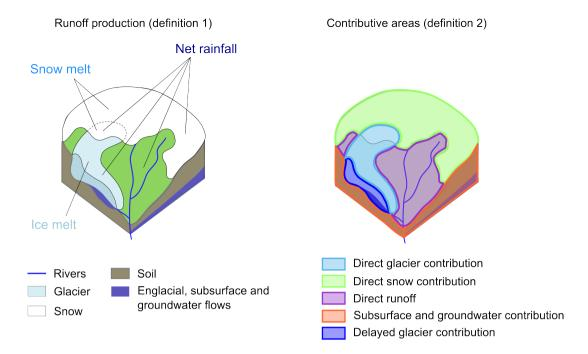
Figure 5. Definitions of the flow components.
