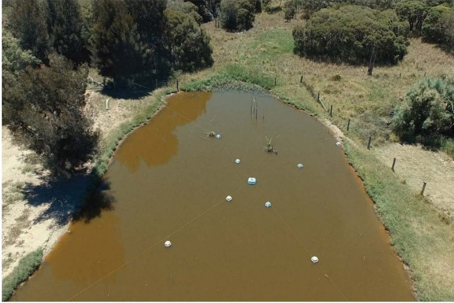
Figure A2A3 . An oblique drone image showing a nine floating chamber deployment setup targeting peripheral and central zones on a stock watering dam (Gatton 3).
