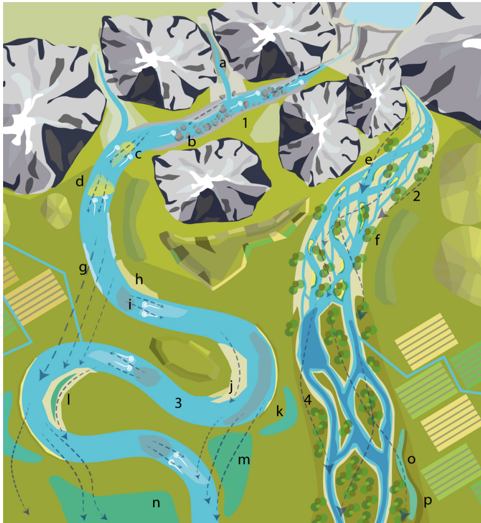
Figure 1. Illustration of catchment complexity: scales and features that influence hyporheic exchange flows. Spatial changes in surface topography, land use and vegetation, drive geomorphological and hydrological changes at valley and reach scale. At catchment scale, variations in surface topography shapes valleys and channel types. Feature 1 refers to confined valleys characterized by straight channels, meandered and braided, and the following floodplain features: scour holes and gravel splays (a). The straight channel presents in-channel cascades (b) geomorphic features. Feature 2 refers to braided channel morphology with multi-thread channel, an undulating floodplain of bars and islands. In-channel geomorphic units are several types of bars (e), such as mid and lateral bars, and vegetated islands (f). Feature 3 represents a sinuous-meandering floodplain with occasional oxbow lakes and backwater swamps (m, n, k) and in channel: longitudinal bar (c), transverse bar (d), counterpoint bar (h), pond-riffle (i), point bar (l), chute channel (j). Feature 4 indicates an anabranching valley with multi-thread channels including abandoned channels (o) and backwater swamps (p). The channel can be quite deep and include islands covered with vegetation.
