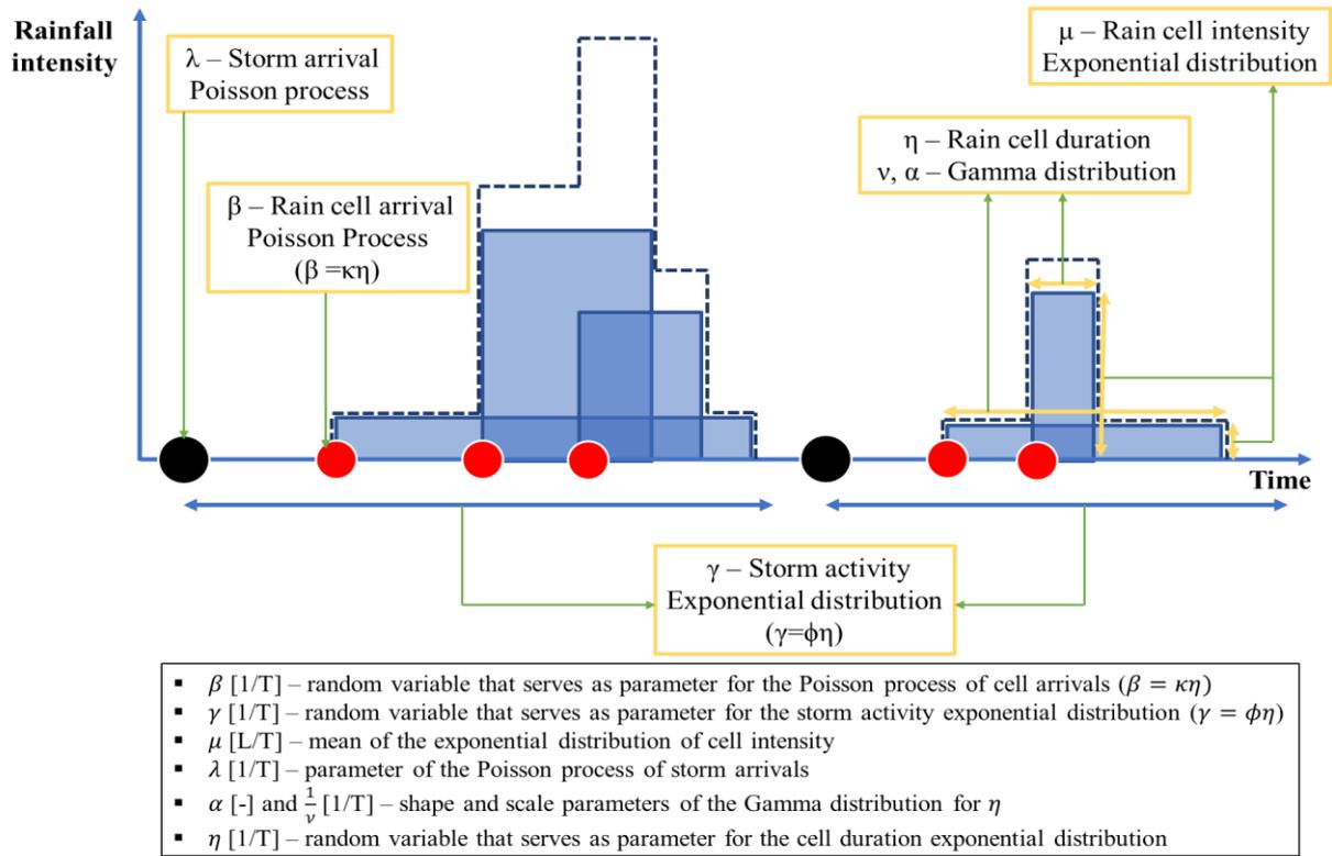
Figure 1: Schematic of the Modified Bartlett-Lewis Rectangular Pulse Model. Blue area represents duration (width) and intensity (height) of each rain cell, respectively. Dashed line represents superposed sum of the rain cell intensities.
