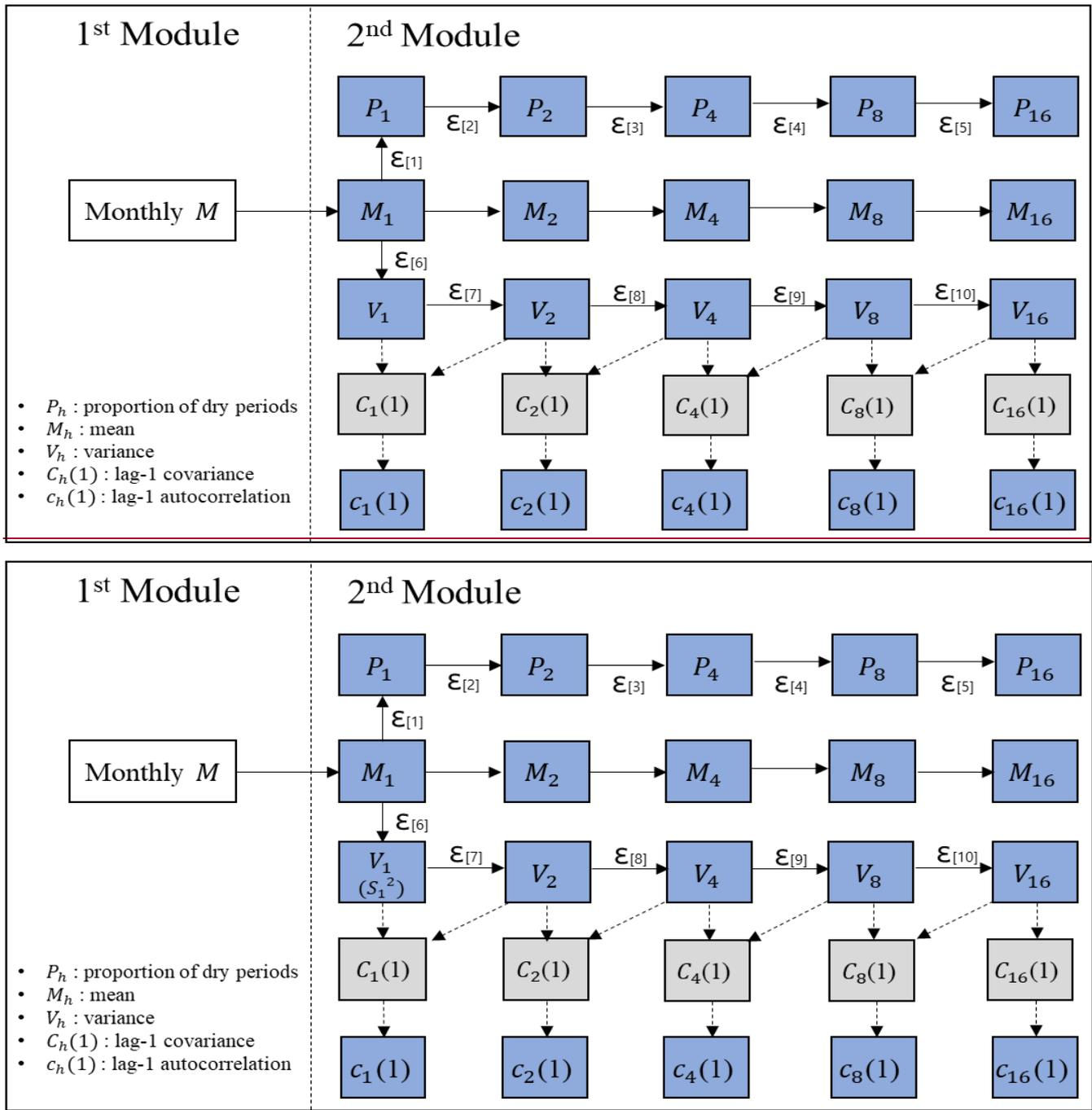
210 **Figure 5: Schematic of the algorithm to generate fine time-scale rainfall statistics. The statistics in the blue boxes are used to calibrate the MBLRP model and the statistics in gray boxes are used to estimate the lag-1 autocorrelation.**
