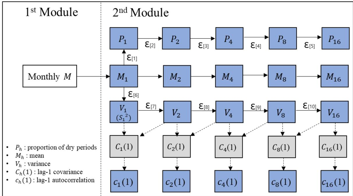
Figure 5: Schematic of the algorithm to generate fine time-scale rainfall statistics. The statistics in the blue boxes are used to calibrate the MBLRP model and the statistics in gray boxes are used to estimate the lag-1 autocorrelation.
