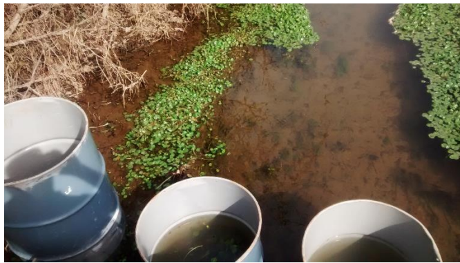
Supplemental Figure 6 – Photo of the small volume MPS being deployed in the Muck section of Goldsboro stream. Emergent vegetation along the banks during March trials resulted in large variability in nitrate decreases over the 24 h experiment.
