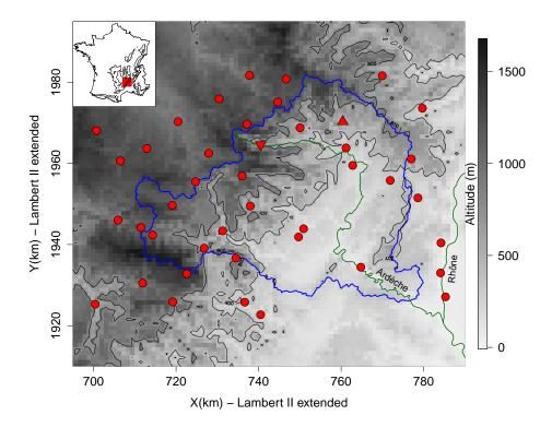
**Figure 1.** Region of analysis. The blue polygon is the Ardèche catchement. The red points show the location of the stations. The upper triangle is the station Antraigues and the lower triangle the station Mayres (both lie at about 500 m.a.s.l.). The background shows the altitude in gray scale (1km raster cells). The top left insert shows a map of France with the studied region in red. The black lines are the 400 and 800 m.a.s.l. isolines.
