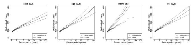
Figure 7. Case of Antraigues when  $G_{s,k}$  is either the extended exponential (eexp), extended Generalized Pareto (egp), lognormal (lnorm) or Weibull (wei) distribution, with S=2 and K=3. The dotted lines show the 95%-envelope of return level estimates over the 100 subsamples. The plain line shows the median estimates. The gray points show the full sample (35 years). Each estimation is based on half these points. Case of the Gamma distribution is shown in the right panel of Figure 5.
