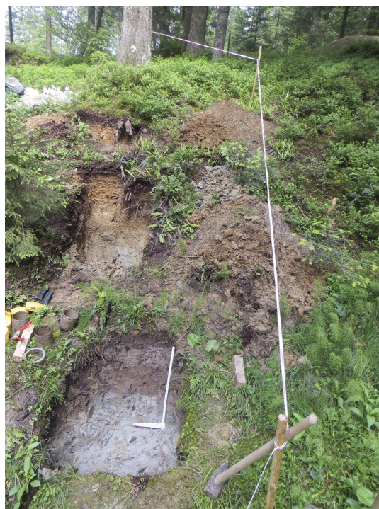
Figure 2. Three analysed soil profiles showing a considerable variation of soil profile characteristics within a short distance. Distance between profiles is 2 m and length of the meter in the lower profile is about 0.6 m.
