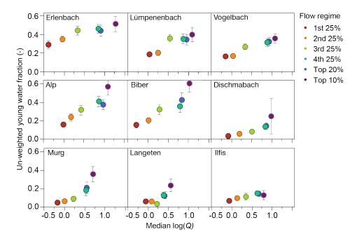
Figure 7: Variation in un-weighted young water fractions with flow regime (log-transformed) for the nine Swiss catchments that have sufficiently long time series of streamwater isotope measurements. Error bars show  $\pm 1$  standard error. The young water fraction increases with discharge differently at different sites, suggesting different degrees of activation of fast flowpaths at high flows.
