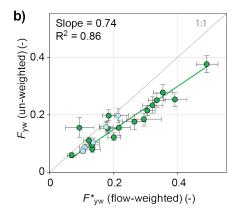
Figure 5: Panel a) compares the seasonal amplitudes of streamwater isotope cycles  $(A_S)$  with and without flow weighting. Highelevation, snowmelt-dominated sites are marked in light blue. Panel b) compares flow-weighted young water fractions  $(F_{yw})$  with un-weighted young water fractions  $(F_{yw})$ . Error bars show  $\pm 1$  standard error. Unweighted young water fractions are roughly 26% smaller than flow-weighted young water fractions across these catchments.
