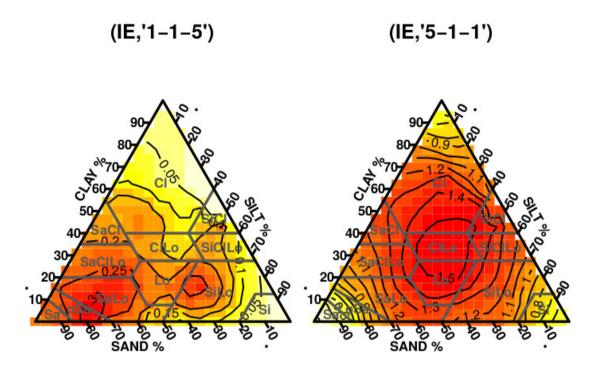
Figure 2. Ternary representations for IE calculated for the soils of the study but using different triplets. The usual clay, silt and sand triplet ('5-1-1') was used at the left and the grouping seven textural fractions into '1-1-5' was used as input for the right.
