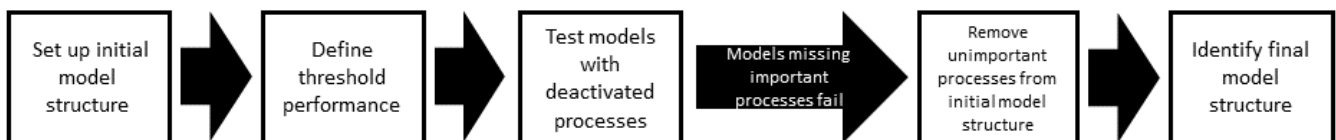
Figure 4: Flow chart for the method of incremental model breakdown
