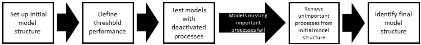
Figure 4: Flow chart for the method of incremental model breakdown
