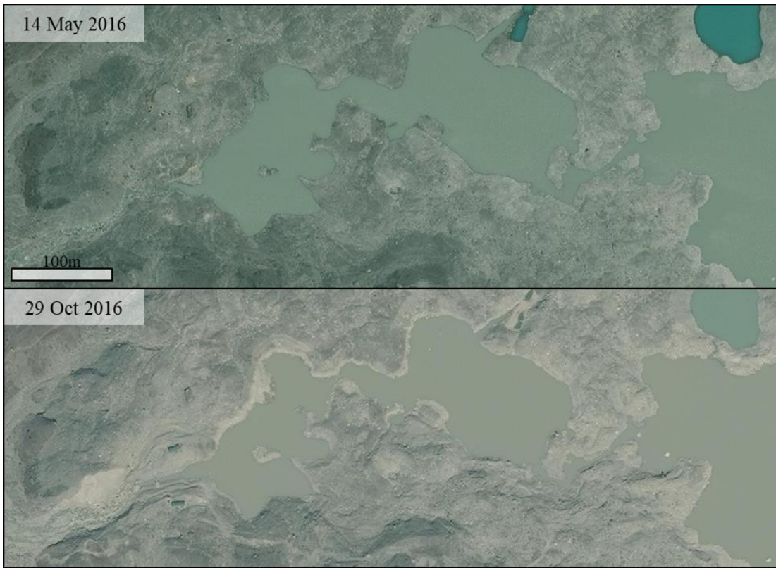
5 Figure 3: WorldView-2 (0.5 m; DigitalGlobe, Inc.) imagery of the lake before (14 May 2016) and after (29 October 2016) the lake lowering project, showing a ring of discoloration around the outlet ponds but not the main lake.
