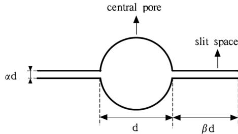
**Figure 2: Pore-space geometry model containing two slit-shaped spaces ( $d$  denotes the diameter of the central pore, and  $\alpha d$  and  $\beta d$  denote the widths and lengths of the slit-shaped spaces, respectively).**
