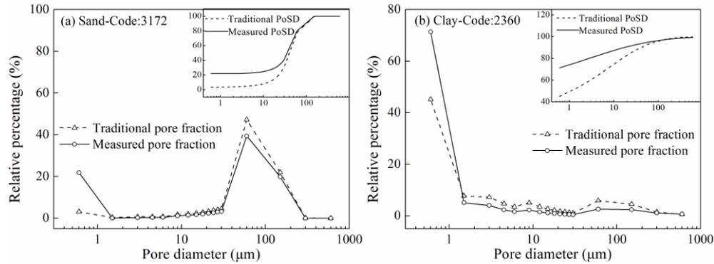
15 **Figure 1: Measured vs. calculated pore volume fraction curves for (a) sand (code: 3172 ) and (b) clay (code: 2360). The measured and calculated PoSDs are ~~embedded~~ embedded in the insets at the tops of the figures.**
