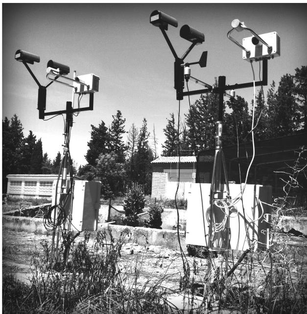
**Figure 1.** Sampling site with four collocated disdrometers
