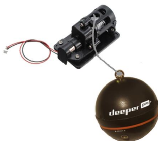
Figure 1. Deeper sonar is connected to a UAV with a wire winch.
