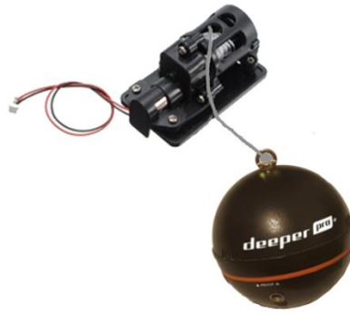
Figure 2. Deeper sonar is connected to a UAV with a wire winch.
