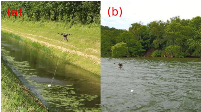
Figure 1. Pictures of the UAV and the tethered sonar. These pictures were retrieved in: (a) Marrebæk Kanal, Denmark. (b) Furesø lake, Sjælland, Denmark. In (b) the drone was flown a few hundreds of meters from the shore and the picture was retrieved using an optical camera onboard an auxiliary UAV (DJI Mavic Pro).
