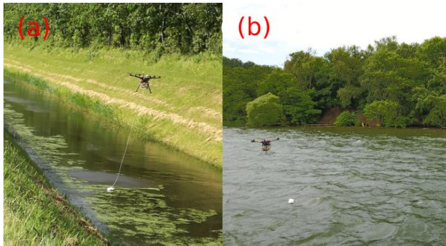
Figure 2. Pictures of the UAV and the tethered sonar. These pictures were retrieved in: (a) Marrebæk Kanal, Denmark. (b) Furesø lake, Sjælland, Denmark. In (b) the drone was flown a few hundreds of meters from the coastline and the picture was retrieved using an optical camera onboard an auxiliary UAV (DJI Mavic Pro).
