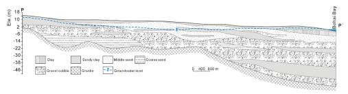
Figure 2. Hydrogeological cross-section of Yang-Dai River Plain (P-P' in Fig. 1) (modified from Han, 1988)
