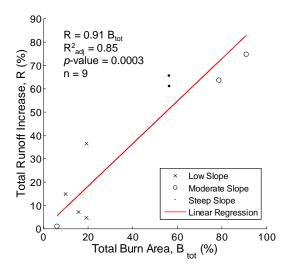
Figure 7: Linear regression model fitted between the total runoff volume increase and total burn area percentage. Catchment slope is categorized as low (slope < 0.30), moderate (0.30  $\le$  slope < 0.40), and steep (slope  $\ge 0.40$ ) for each sub-basin.
