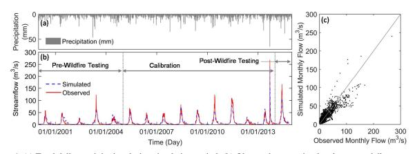
Figure 4: (a) Total daily precipitation during simulation period. (b) Observed versus simulated average daily streamflow hydrographs. (c) Observed versus simulated average daily streamflows scatter plot.
