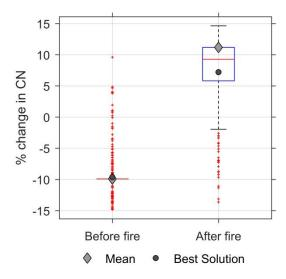
Figure 3: Boxplots showing the range of % change in CNs for before and after fire conditions (the boxes show the range of values between 25th and 75th percentile; the whiskers show the 0.5 and 99.5 percentile).
