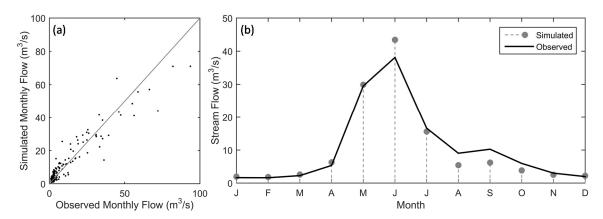
Figure 10: (a) Scatter plot of simulated versus observed monthly streamflows and (b) the observed versus simulated average monthly streamflows for the simulation period.
