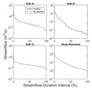
Figure 9: Flow-duration curves for select sub-basin as well as the entire study watershed. Subbasin area and percentage of burned area for subbasins 30; 35; 19 and study watersheds are: 11 km2, 79%; 269 km2, 16%; 90 km2, 10% and 2,732 km2, 14% respectively.
