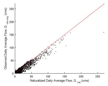
Fig. A5. CDWR naturalized daily average streamflow versus observed daily average streamflow with 1 to 1 reference line.
